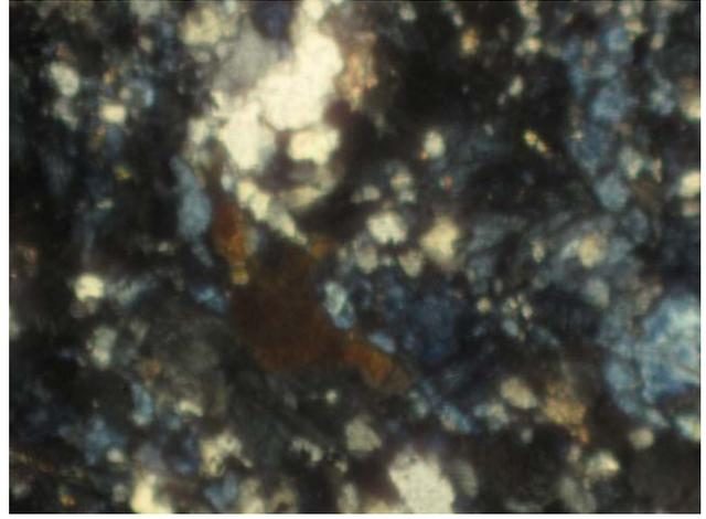
**Fig. 10.** An intermixing of off-white (medium to fine grained) scheelite, gray quartz, bluish clinzoisite, brownish red biotite and black magnetite in XPL (80×)
