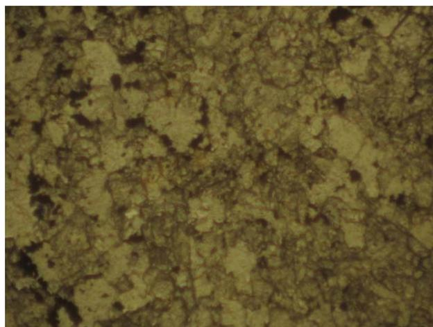
**Fig. 5.** Off-white to yellowish brown (angular to sub-rounded) grains of scheelite embedded in quartz and clinzoisite grains in plane polarized light (PPL) (40×)
