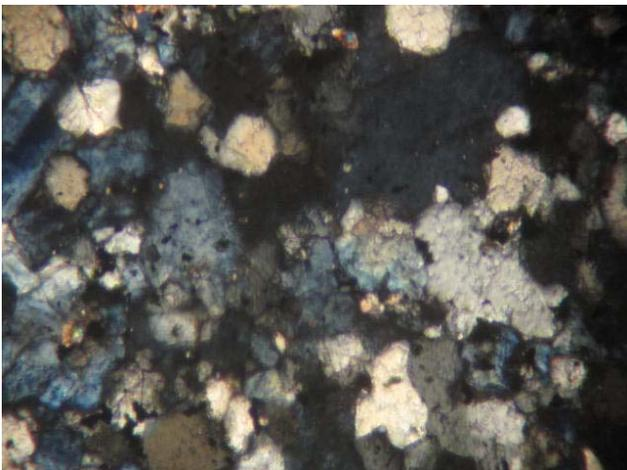
**Fig. 7.** Another view under high magnification (80×) shows grayish white to yellowish brown scheelite crystals in XPL
