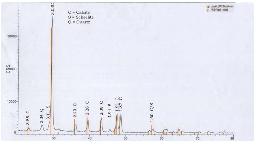
**Fig. 3.** X- Ray Diffractogram (XRD) of Besti Gole tungsten ore, district Chitral, KPK Province, Pakistan
