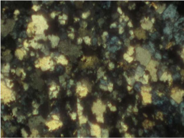
**Fig. 6.** Same photomicrograph under cross polarized light (XPL) (40×) showing light bluish clinzoisite matrix and yellowish to light brown crystals of scheelite in gray quartz
