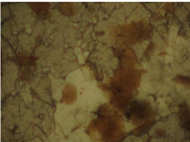
**Fig. 8.** Magnetite grains looks gray with brownish tint in PPL (80×)
