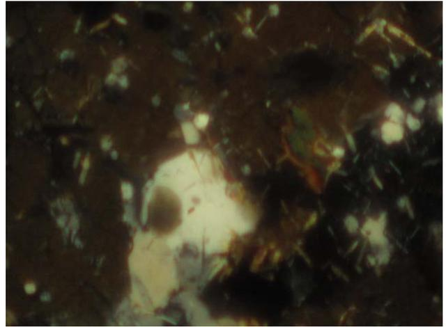
**Fig. 9.** Magnetite grains observed dark black under XPL in same photomicrograph (80×)
